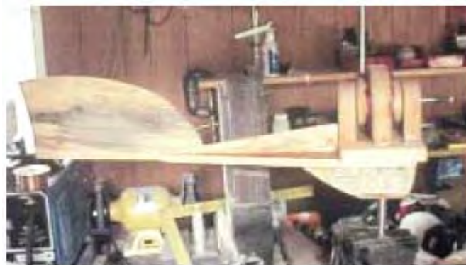
Almost ready—the wooden frame and tail are attached.
